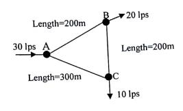
Assume that RL of points A, B and C is same. The pressure available at A is 15kg/cm<sup>2</sup> and the minimum pressure required at B and C is 1.5 Kg/cm<sup>2</sup>.
