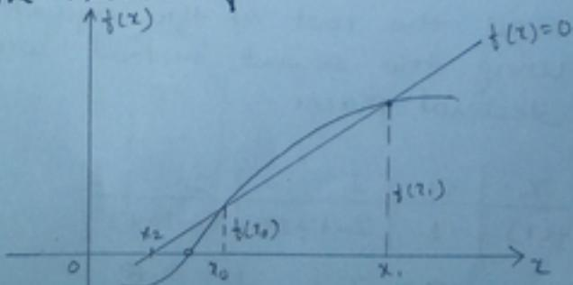
Secant method, like the false position and bisection methods, uses two initial state estimates but does not require that they must bracket the root. Here, also the graph of the function  $y = f(x)$  is approximated by a secant line but at each iteration, two most recent approximations to the root are used to find the next approximation. Also it is not necessary that the interval must contain the root.
