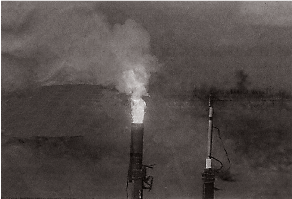
Fig. 18.1 A hygroscopic cartridge being burnt to demonstrate the process of cloud seeding, which was inaugurated at the Jakkur airfield in Bangalore on Monday-Aug. 2003
