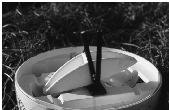
Figure 2.10 The insides of a tipping-bucket rain gauge. The 'buckets' are the small white, triangular reservoirs. These are balanced and when full they tip over bringing the black arm past the other stationary arm. In doing so a small electrical current is passed to a data logger.
