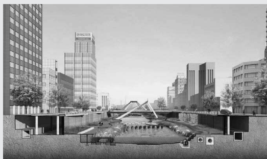
Figure 8.15 Schematic diagram of Cheonggyecheon restoration project, showing infrastructure as well as the river.
