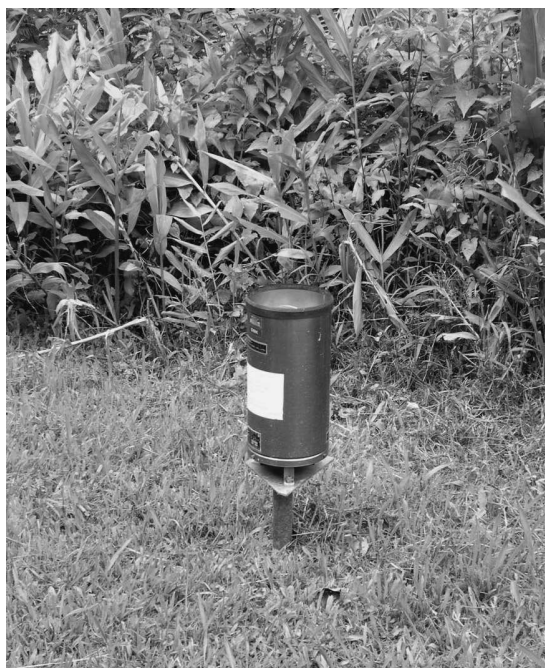
Figure 2.5 A rain gauge sitting above the surface to avoid splash.
