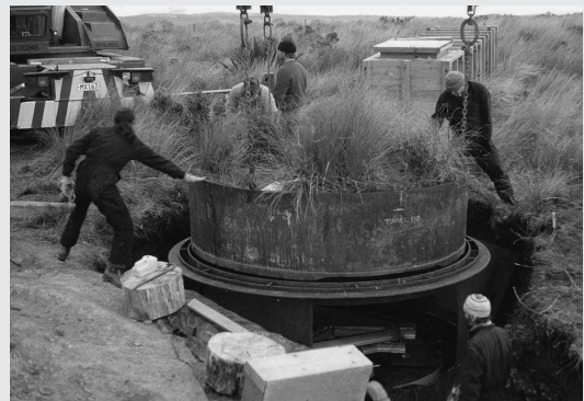
Figure 3.5 Large weighing lysimeter at Glendhu being installed. The weighing mechanism can be seen underneath.
