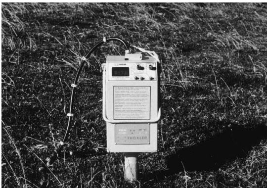
Figure 4.10 A neutron probe sitting on an access tube. The black cable extends down into the tube with the source of fast neutrons (and counter) at the tip.
