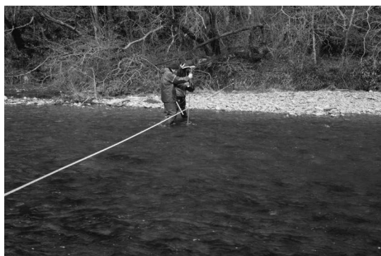
Figure 5.7 Flow gauging a small stream.
