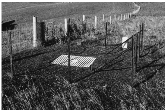
Figure 2.6 Surface rain gauge with non-splash surround.
