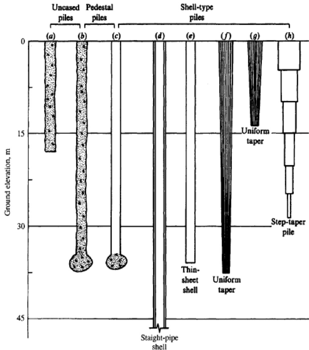
**Figure 16-7** Some common types of cast-in-place (patented) piles: (a) Commonly used uncased pile; (b) Franki uncased pedestal pile; (c) Franki cased pedestal pile; (d) welded or seamless pipe; (e) Western cased pile; (f) Union or Monotube pile; (g) Raymond standard; (h) Raymond step-taper pile. Depths shown indicate usual ranges for the various piles. Current literature from the various foundation equipment companies should be consulted for design data.
