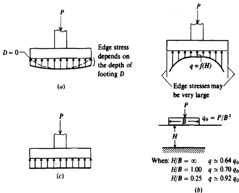
**Figure 8-2** Probable pressure distribution beneath a rigid footing. (a) On a cohesionless soil; (b) generally for cohesive soils; (c) usual assumed linear distribution.
