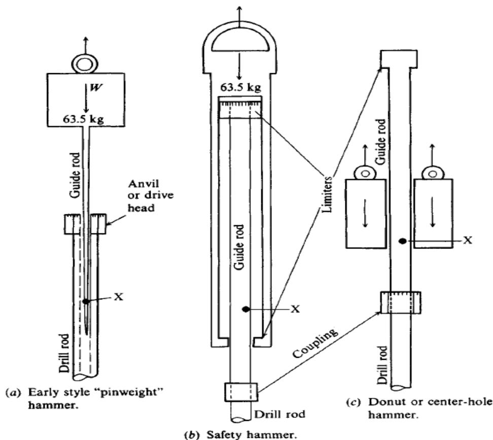
**Figure 3-7** Schematic diagrams of the three commonly used hammers. Hammer (b) is used about 60 percent; (a) and (c) about 20 percent each in the United States. Hammer (c) is commonly used outside the United States. Note that the user must be careful with (b) and (c) not to contact the limiter and "pull" the sampler out of the soil. Guide rod X is marked with paint or chalk for visible height control when the hammer is lifted by rope off the cathead (power takeoff).
