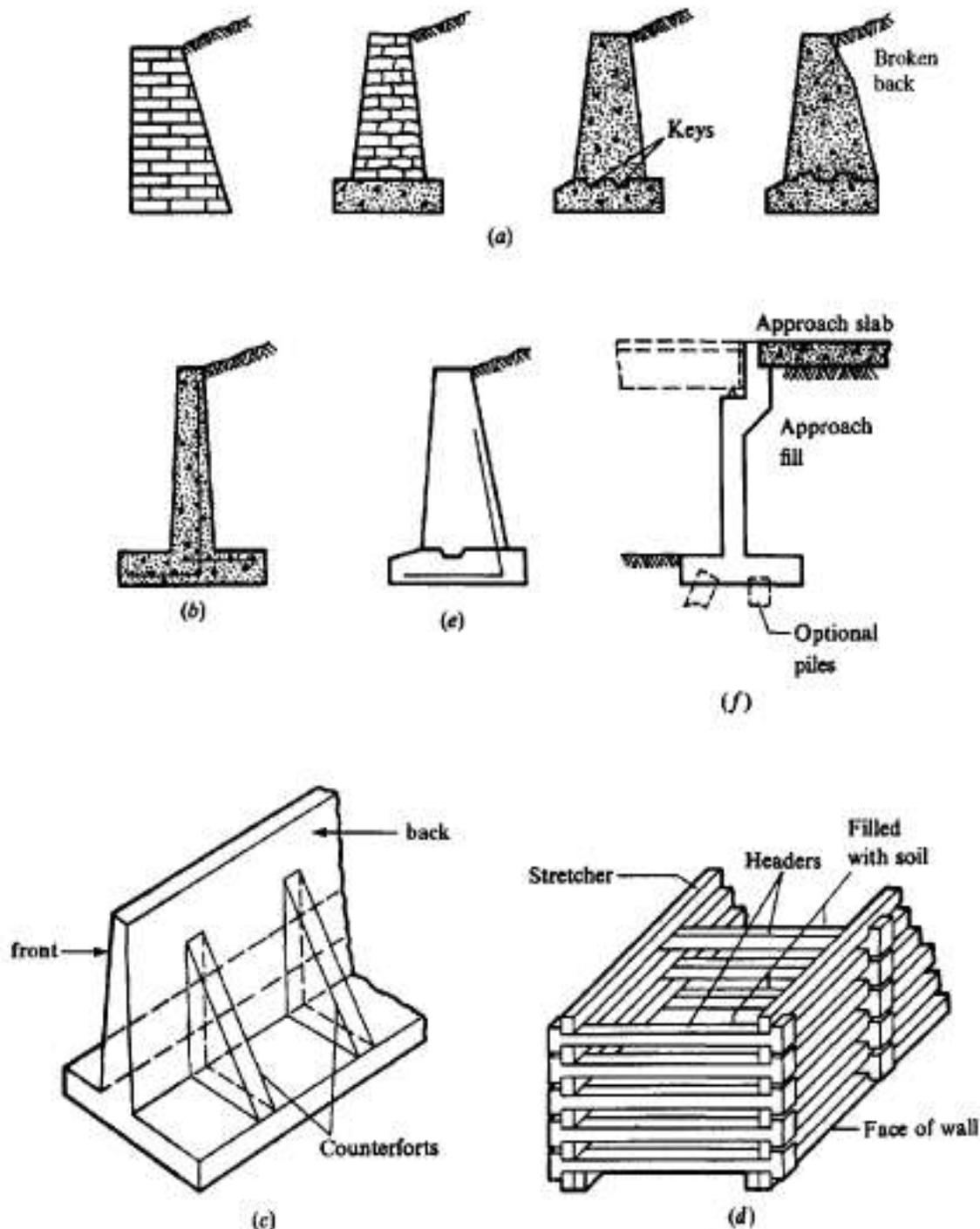
**Figure 12-9** Types of retaining walls. (a) Gravity walls of stone masonry, brick, or plain concrete—weight provides stability against overturning and sliding; (b) Cantilever wall; (c) Counterfort, or buttressed wall—if backfill covers the counterforts the wall is termed a counterfort; (d) Crib wall; (e) Semigravity wall (uses small amount of steel reinforcement); (f) Bridge abutment.
