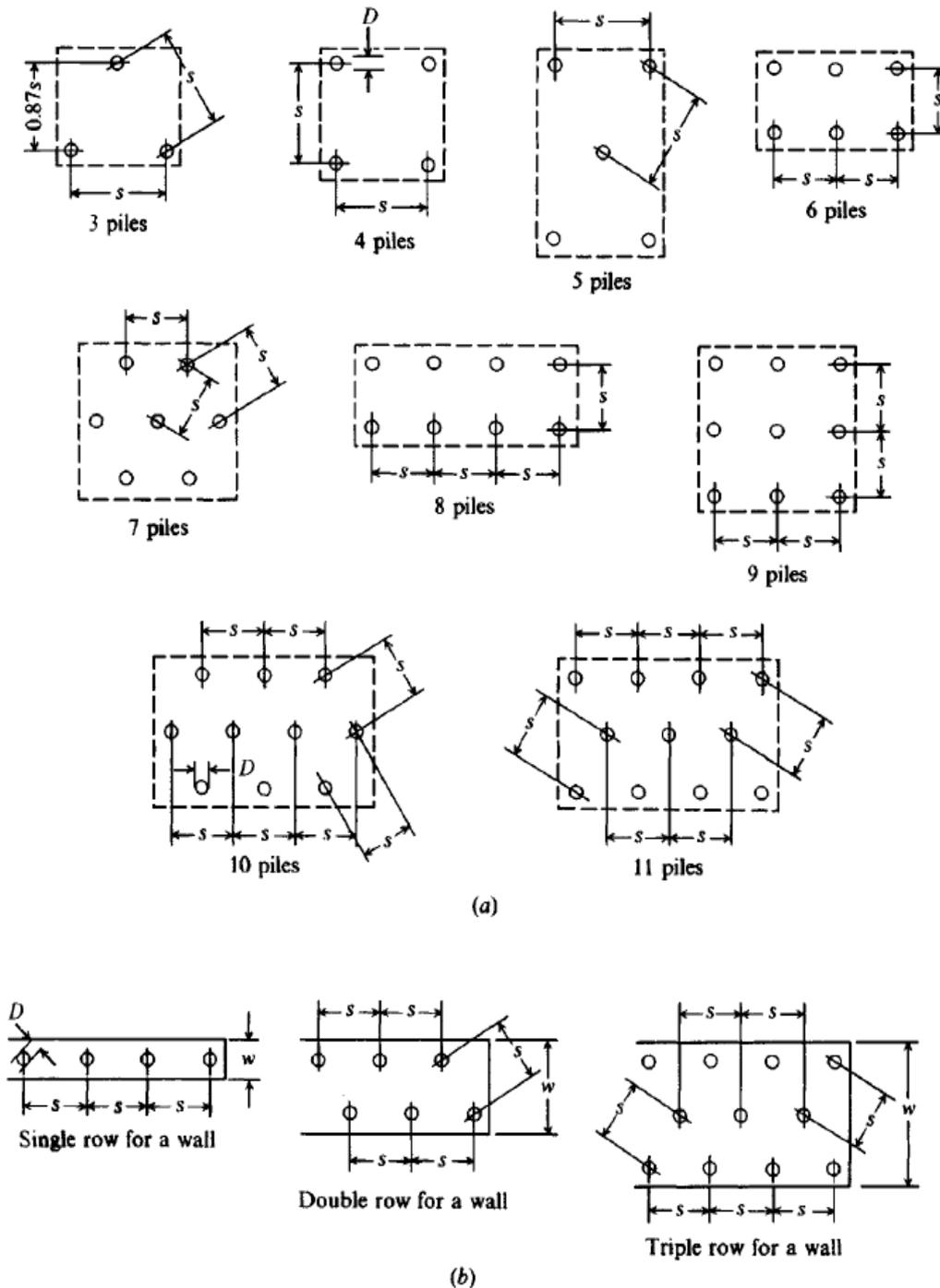
Figure 18-1 Typical pile-group patterns: (a) for isolated pile caps; (b) for foundation walls.
