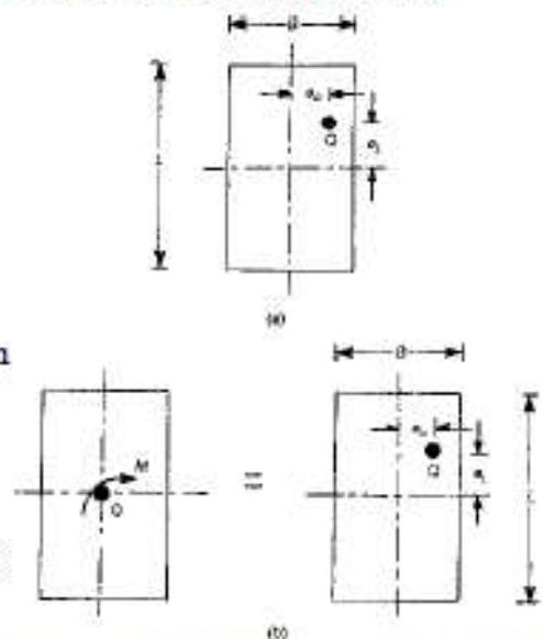
Figure 1-5 Eccentric load on rectangular foundation
