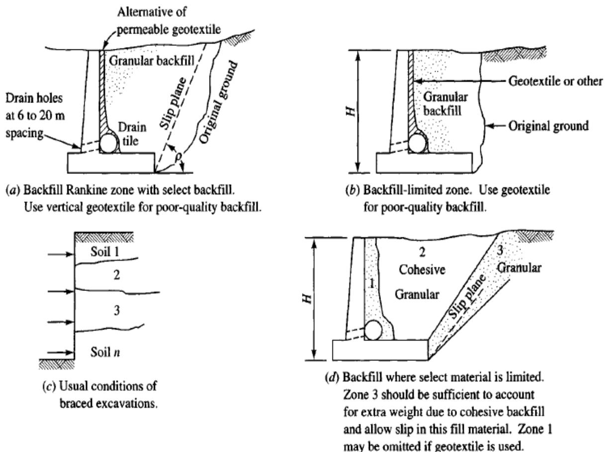
**Figure 11-12** Various backfill conditions. The longitudinal collector (or drain) pipe is optional.
