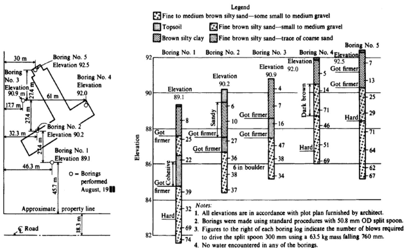
Figure 3-37 A method of presenting the boring information on a project. All dimensions are in meters unless shown otherwise.
