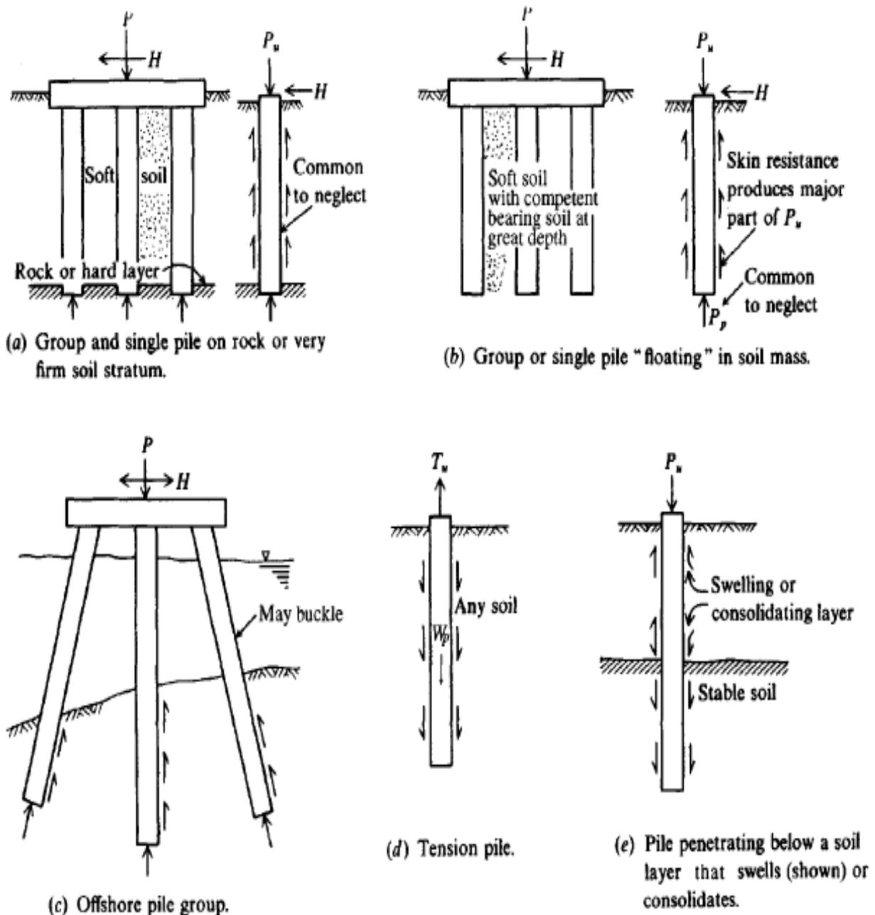
**Figure 16-1** Typical pile configurations. Note that, whereas analysis is often for a single pile, there are usually three or more in a group. Typical assumptions for analysis are shown. Lateral load  $H$  may not be present in (a) or (b).
