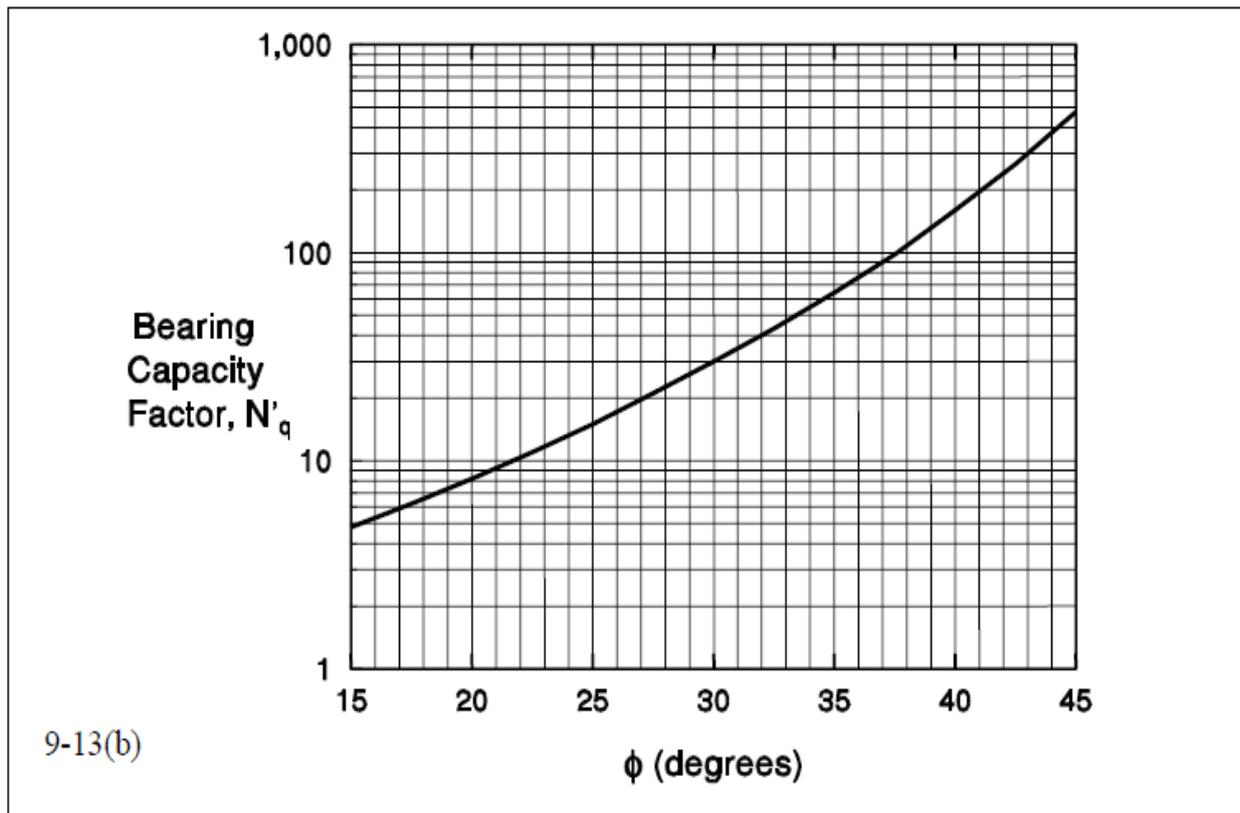
Figure 9-13. Chart for estimating  $\alpha_t$  coefficient and bearing capacity factor  $N'_q$  (FHWA, 2006a).
