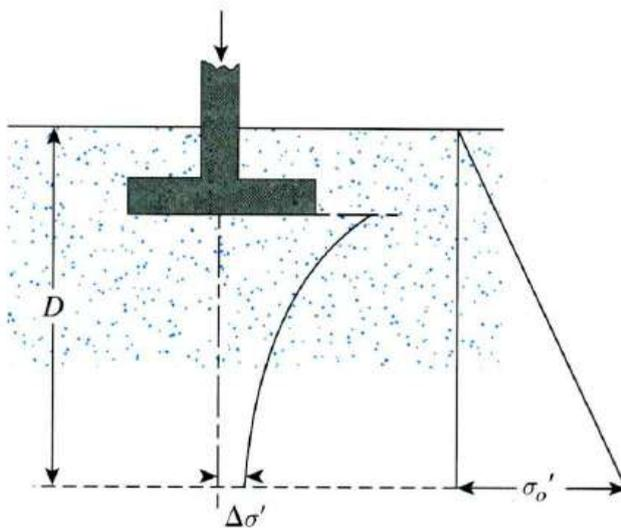
**Figure 2.9** Determination of the minimum depth of boring
