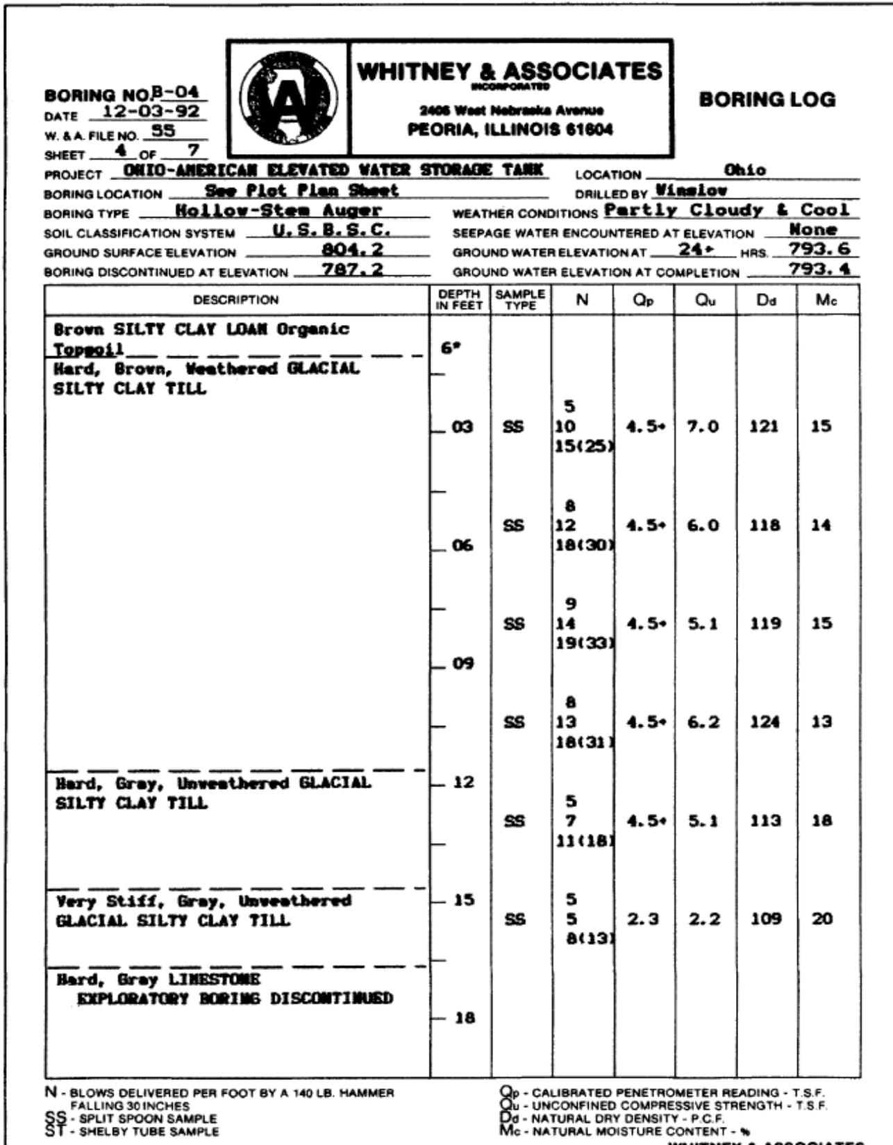
Figure 3-38 Boring log as furnished to client.  $N$  = SPT value;  $Q_p$  = pocket penetrometer;  $Q_u$  = unconfined compression test;  $D_d$  = estimated unit weight  $\gamma_s$ ;  $M_c$  = natural water content  $w_N$  in percent.
