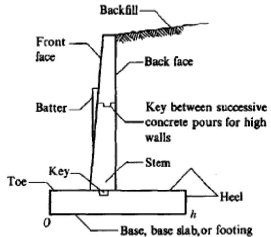
**Figure 12-11** Tentative design dimensions for a cantilever retaining wall. Batter shown is optional.
