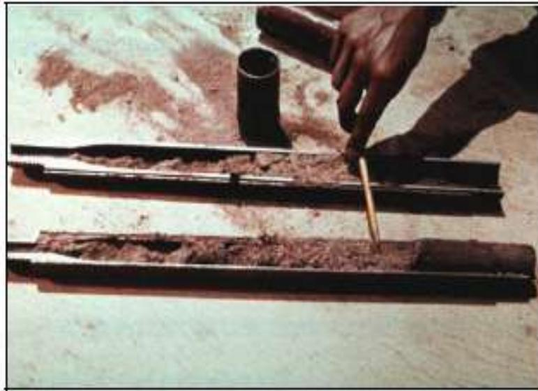
**Split Barrel Sampler: Open sampler with soil sample and cutting shoe.**
