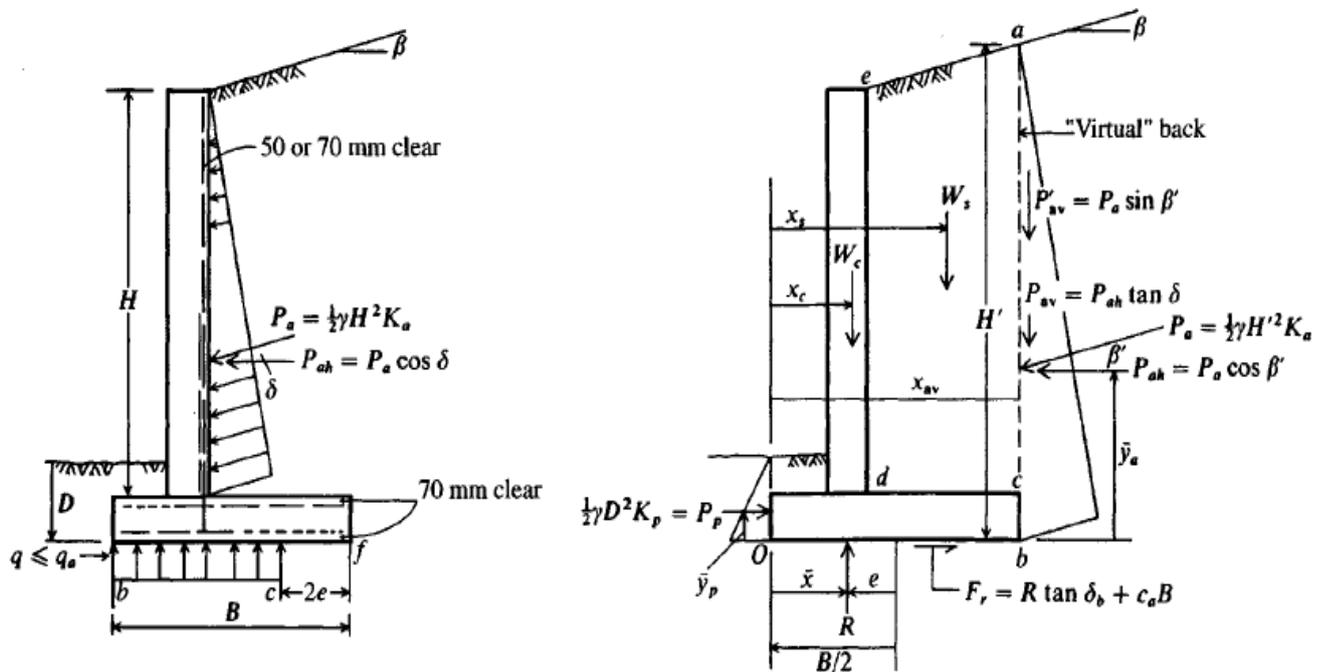
(a) Wall pressure to use for shear and bending moment in stem design. Also shown is bearing capacity pressure diagram based on Fig. 4-4 using  $B' = b - 2e$  and  $L = L' = 1$  unit.
