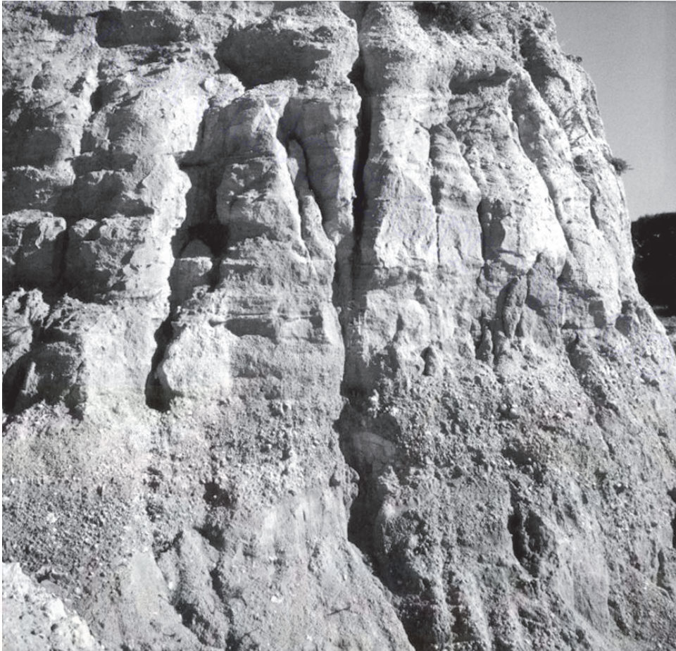
Figure 5.5 A photograph of the face of a sand and gravel pit showing lenses and layers of sand and gravel particles of different sizes. (Aller gravels, Devon.)
