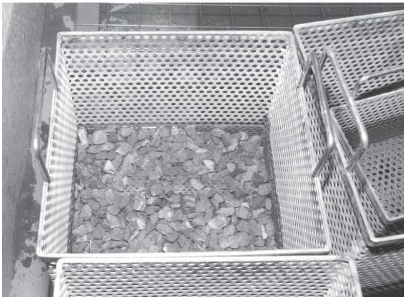
Figure 8.6 Aggregate soaking in saturated magnesium sulfate solution during soundness testing.
