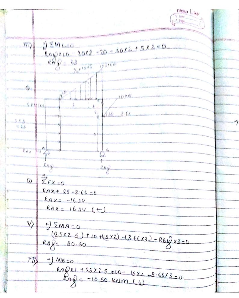
Axial force shearing force and bending " :!! :!!
